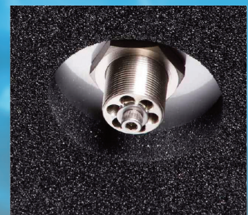
Fiber wave guide as seen from inside the Ka Shield cabinet.
