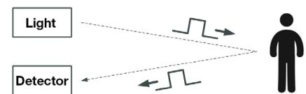
Schematic representation of ToF technology: Light is emitted (diode), this hits an object (person), the light is reflected and then detected in the sensor. The distance of the object to the sensor can then be determined from this data.
