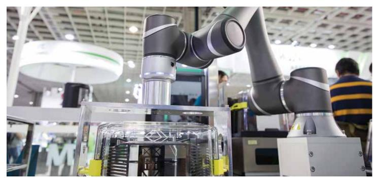
Collaborative robots generally support lighter payloads than standalone robots, but they offer greater flexibility.
