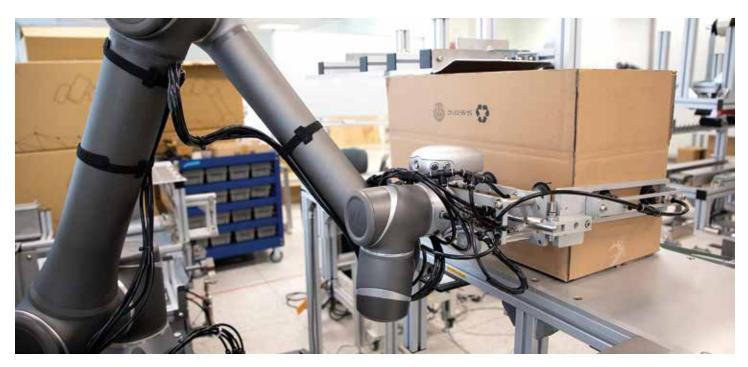
Collaborative robots provide a highly flexible solution for packaging applications.
